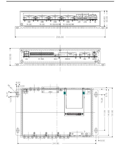
Figure 1.1: Chassis Dimensions
